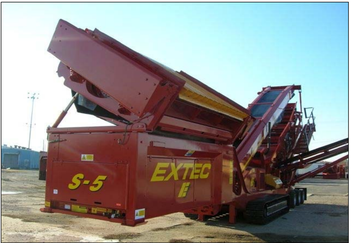
Remote tipping vibrating grid
