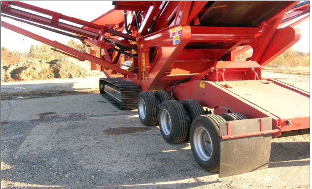
Hydraulically raises machine onto bogie
