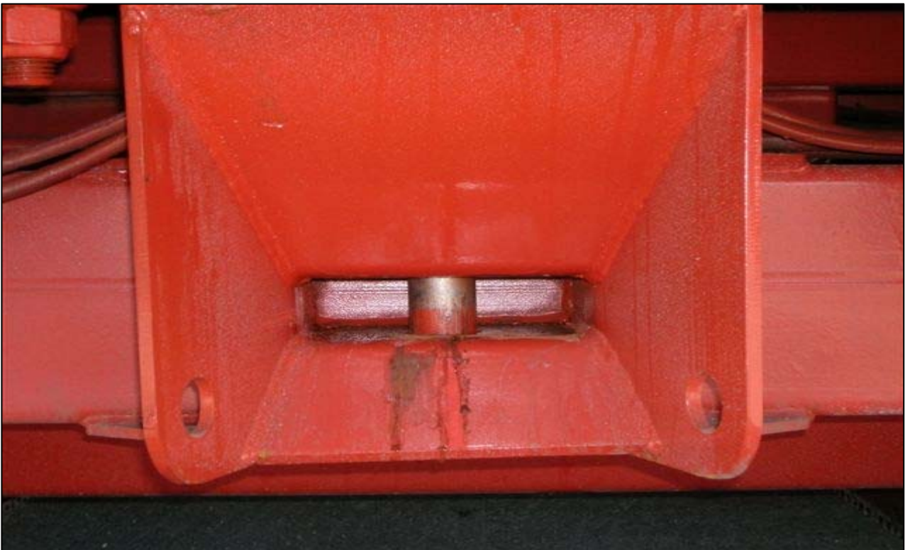
Hydraulic hitch pin ensures attachment of bogie.
