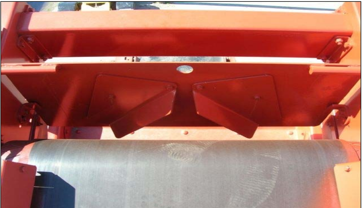
Adjustable swinging spreader plate ensures even spread of materials across the screen box
