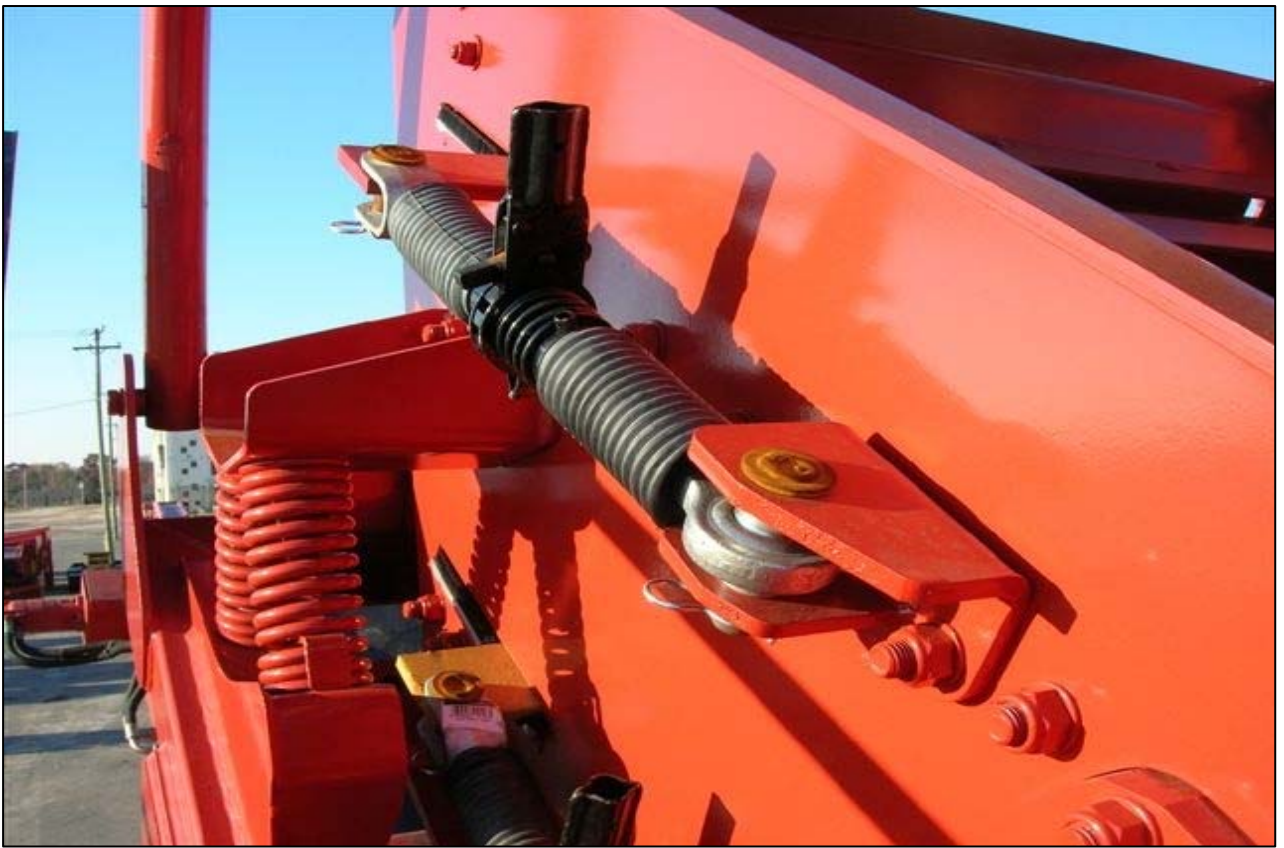
Manual ratchet system for quick mesh change
