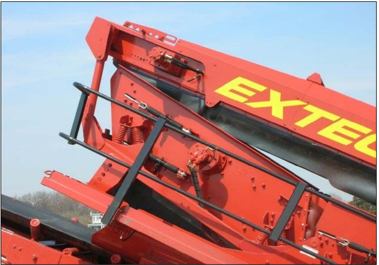
First screen box max angle 37°
