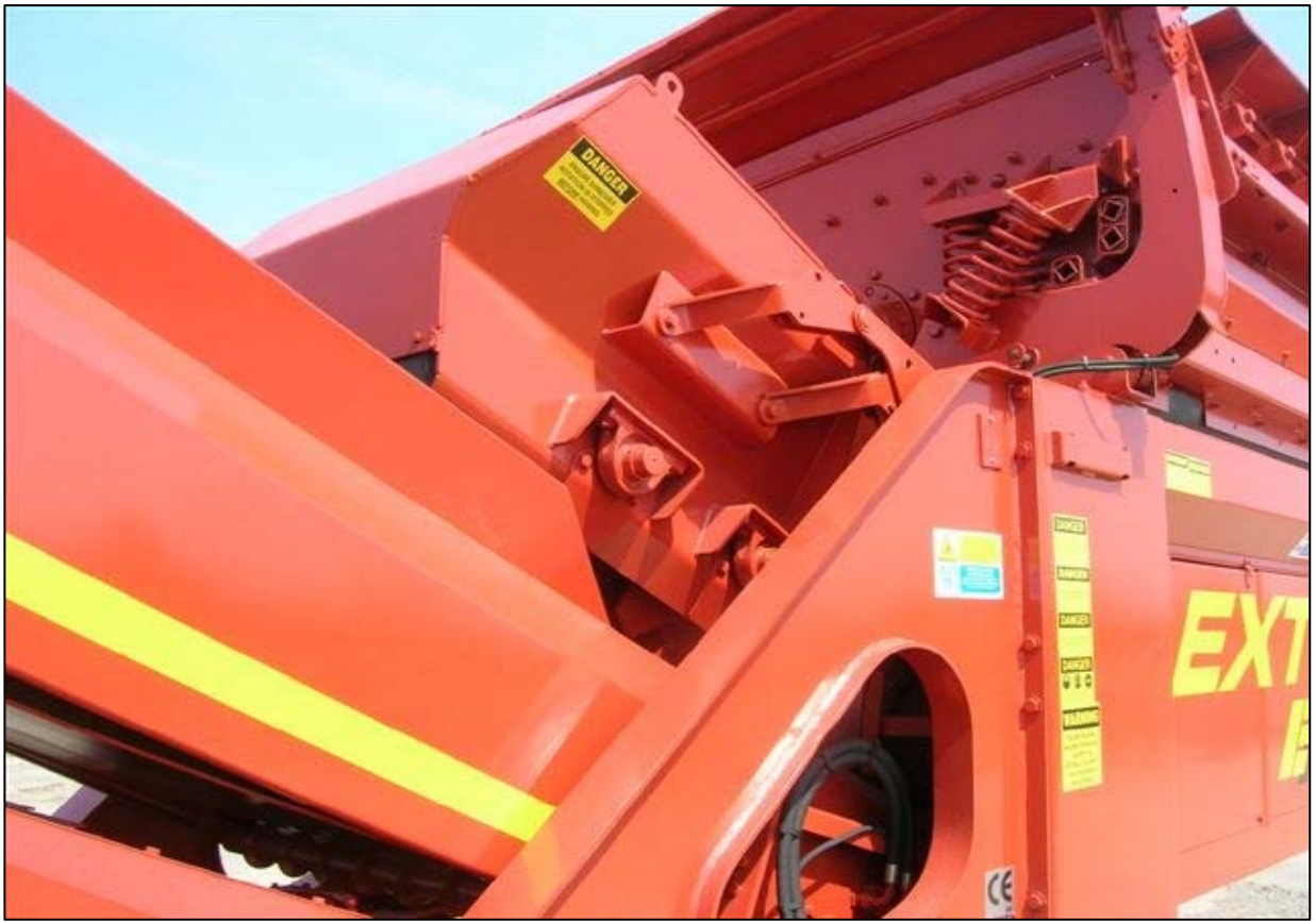
Optional shredder hydraulic raise & lower
