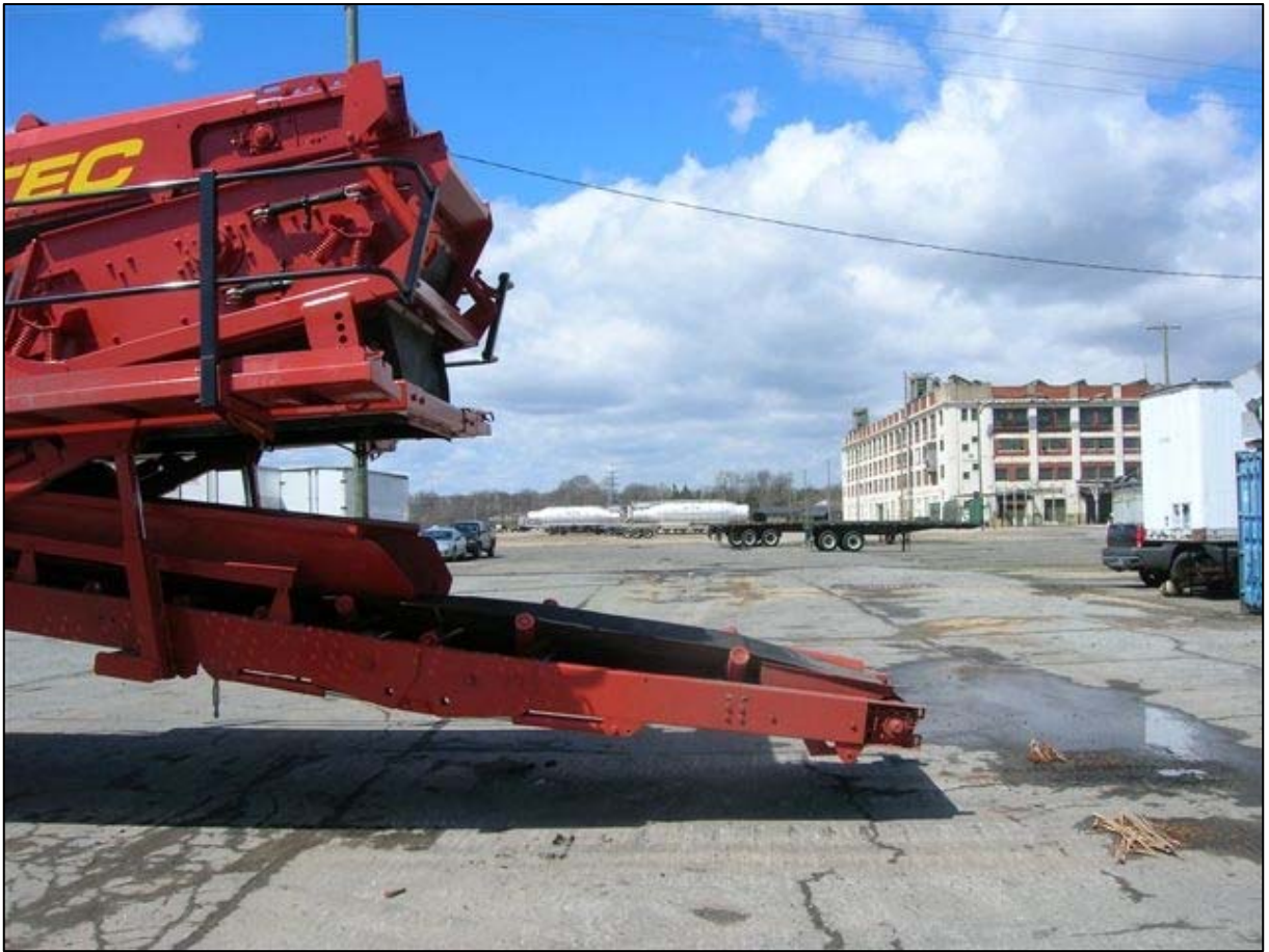
Tail conveyor lowers to facilitate easy mesh change
