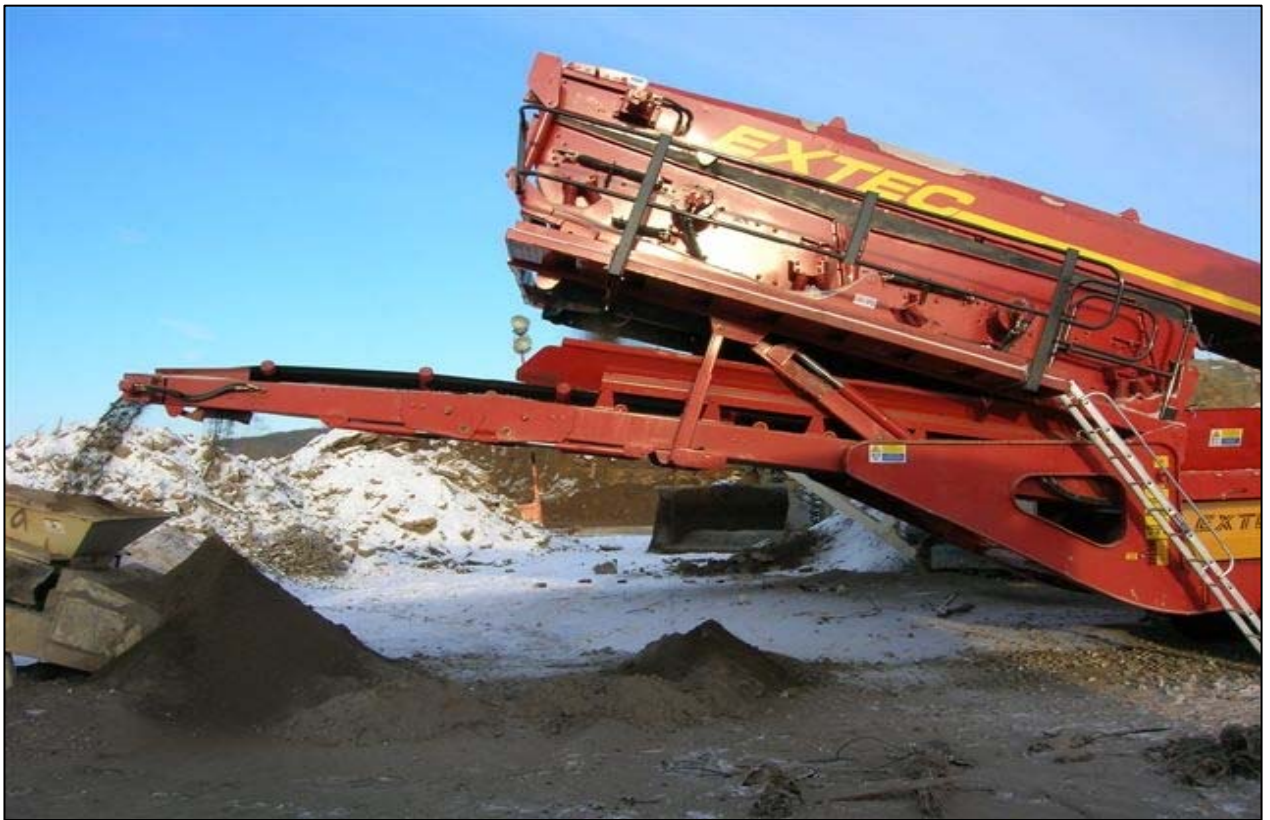
Tail conveyor lowers to aid feeding of conveyors
