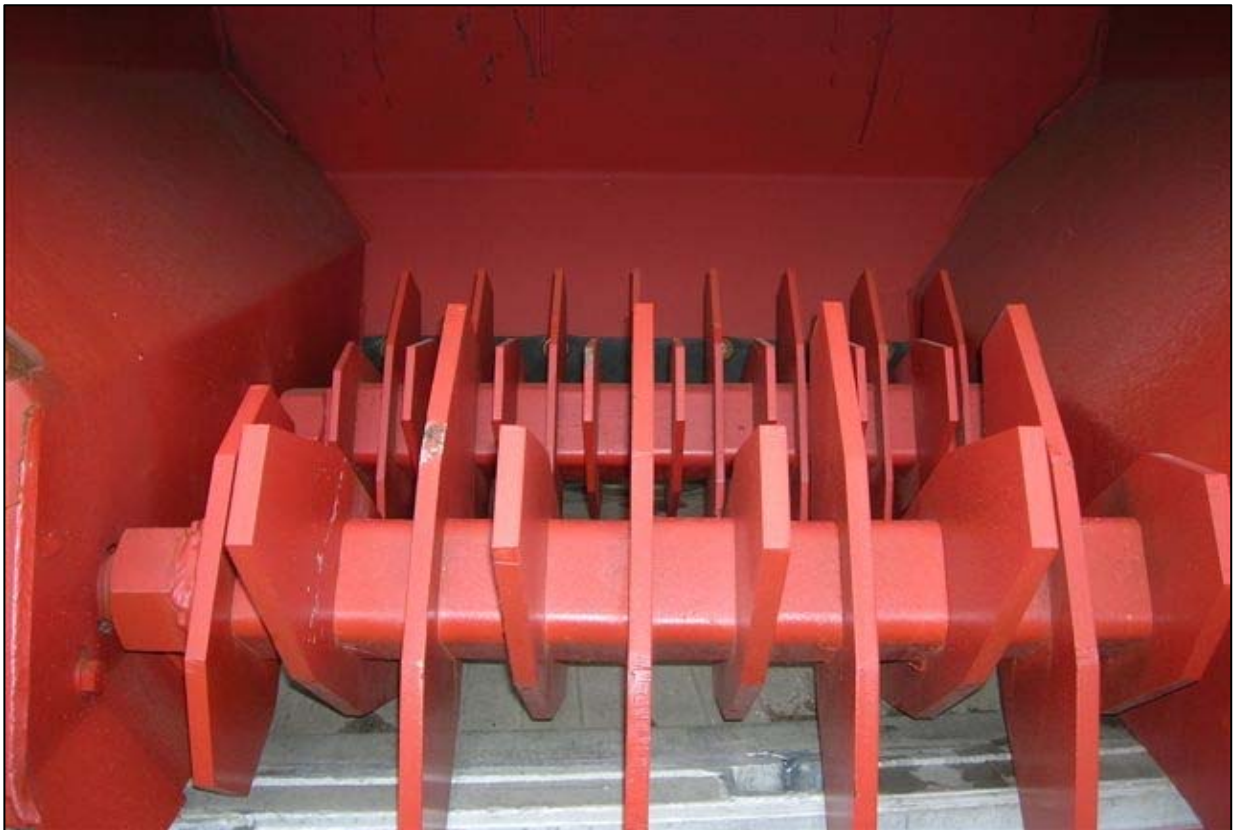
Hydraulic drive shredder, double shafts, fixed blade 650rpm
