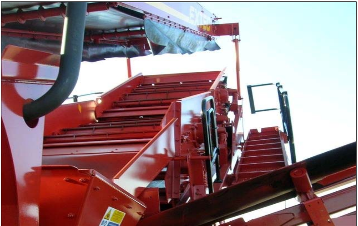
Hydraulic raise of main conveyor ensures maximum access
