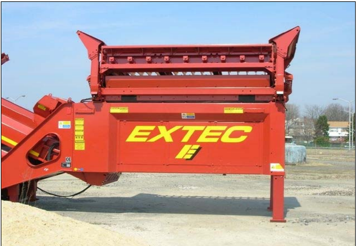
Hydraulic hopper raise - lower legs
