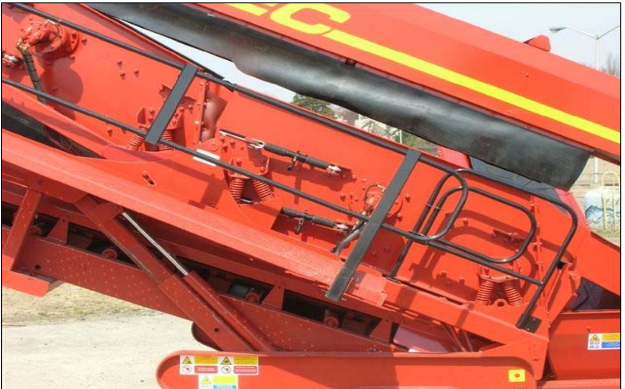
Second screen box max angle 27°
