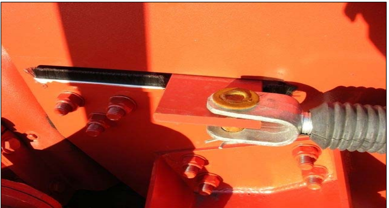
Screen box design allows for mesh change without the need to remove spring bar
